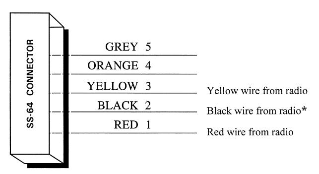
Notes: \* If you want to turn the encoder on and off, use the violet wire in the radio instead of the black wire for the ground connection. This will allow the encoder to be turned on or off with the tone switch on the squelch control
