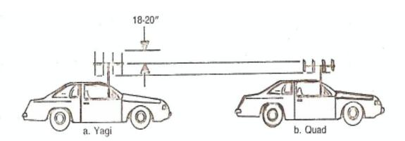
Figure 4.5 A full sized 2 meter quad is much shorter than a similar Yagi
