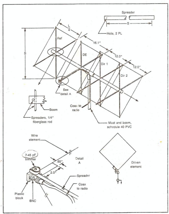
Fig. 4-6. Design details of a strung wire quad, shown vertically polarized. Design center frequency is 147 MHz.
