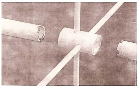
Figure 4.7 The Collapsible version boom is knotched for proper alignment
